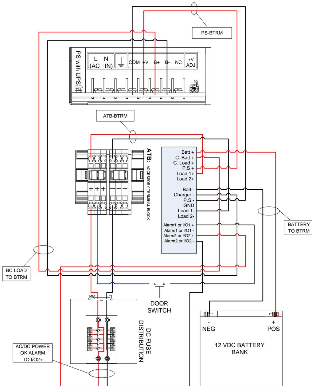
Figure 1: UPS Enclosure System with BTRM.
